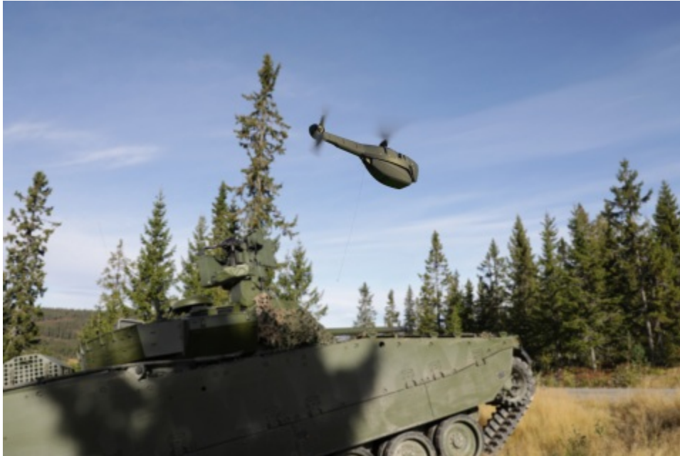
FLIR Black Hornet Vehicle Reconnaissance System enables autonomous operation of Black Hornet 3 UAV from within military vehicles. (Photo: Business Wire)
